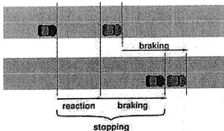
The stopping distance depends on the reaction time of the combined object detection system and the onboard automatic breaking system, the speed of travel, and the road condition, see the figure below.
