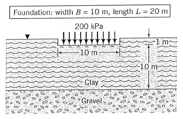
Figure 5: The vertical section through a building foundation.
