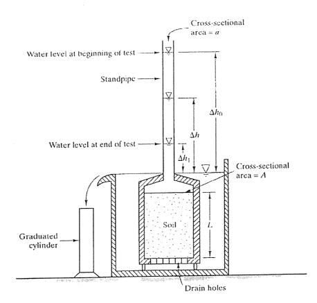
Figure 3: The falling head permeameter test apparatus.
