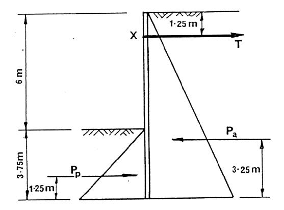
Figure 4: The anchored sheet-pile wall.
