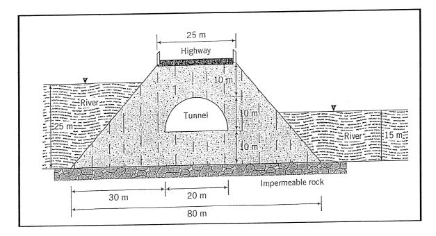
b) Determine the uplift force per unit length at the base of the tunnel.
