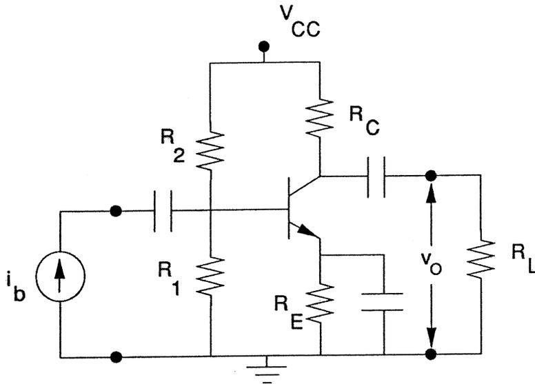
**Figure 1 Transistor Circuit**
