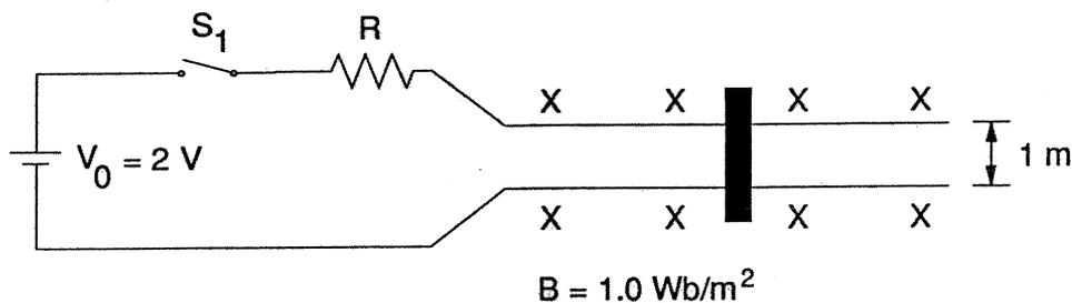
Figure 3 Top View of Linear dc Machine
