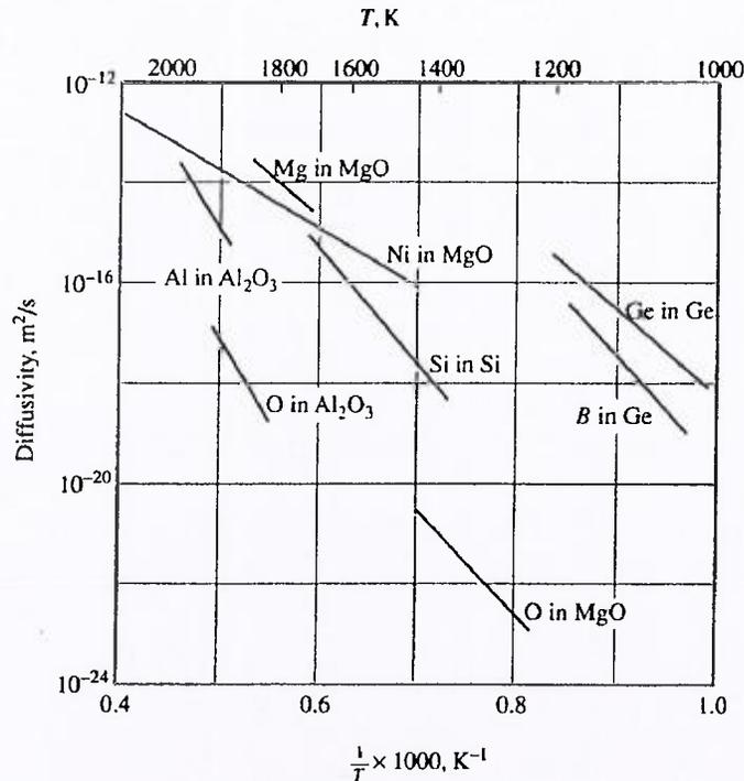
Fig 1 Diffusivity data for some non-metallic systems
