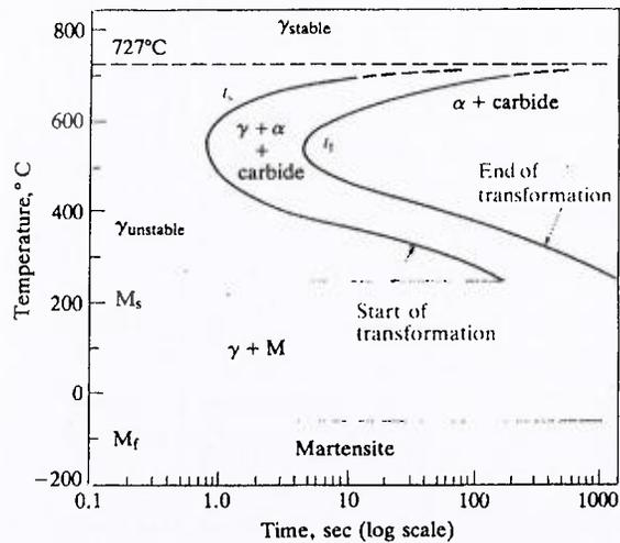
Fig 2 Isothermal diagram for a 0.8% carbon steel
