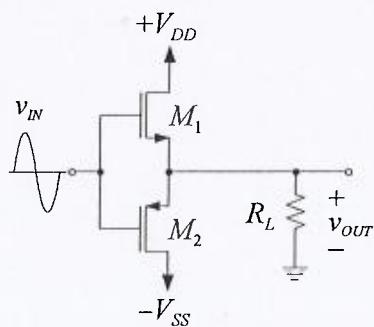
Given:  $K = 500\text{ mA/V}^2$ ,  $V_{TH} = 1.0\text{ V}$ ,  $R_L = 8\Omega$  and  $|V_{DD}| = |V_{SS}| = 10\text{ V}$ .
