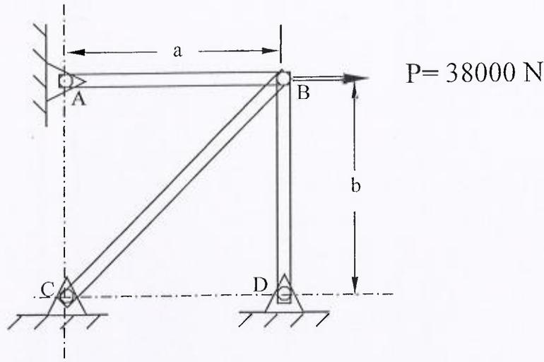
2. Determine the magnitude and direction (up or down) of the force  $P$  if the displacement at A is not to exceed 7 mm (down). Take  $E = 180 \text{ GPa}$  and  $I = 805 \times 10^6 \text{ mm}^4$ .
