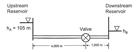
Figure 2. Schematic of water transmission system.
