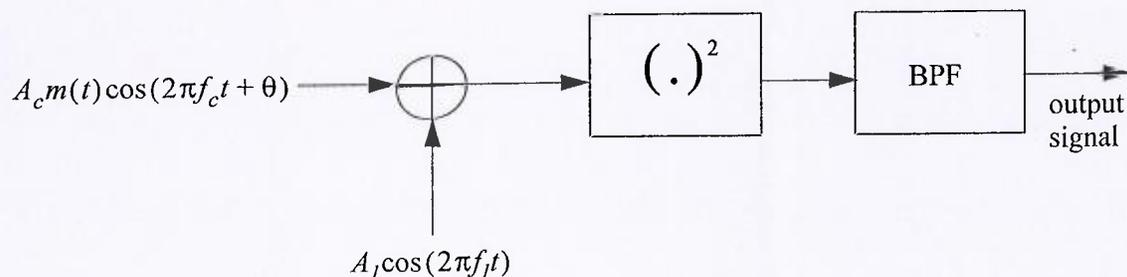
The band-pass filter has a center frequency  $f_i = |f_c - f_l|$  (also known as the intermediate frequency, IF). Assume that the message bandwidth of the input signal  $m(t)$  is equal to  $B$  Hz.
