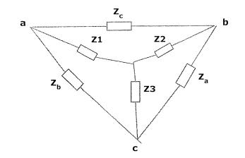
$$Z_{1} = \frac{Z_{b}.Z_{c}}{Z_{a} + Z_{b} + Z_{c}} \qquad \qquad Z_{2} = \frac{Z_{a}.Z_{c}}{Z_{a} + Z_{b} + Z_{c}} \qquad \qquad Z_{3} = \frac{Z_{a}.Z_{b}}{Z_{a} + Z_{b} + Z_{c}}$$
