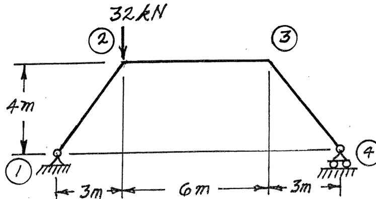
(18) 4. For the trusses shown below, calculate the forces in the members that are listed. For each force, indicate whether it is tension or compression.
