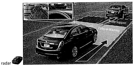
You are using a radar detector to measure the distance of the car in front of you, and a warning will be issued to you when your car is within 15 meters from the car ahead, so that you can stop your vehicle by applying the brakes manually. If you are within 10 meters to the car ahead, the collision avoidance system will deploy automatic break to stop your car.
