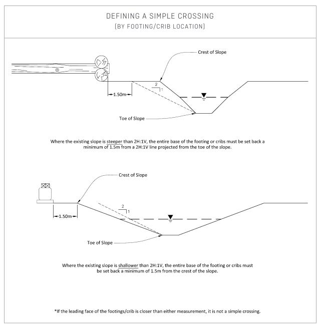
*Figure D - 1: Illustration of a Simple Crossing Slope*
