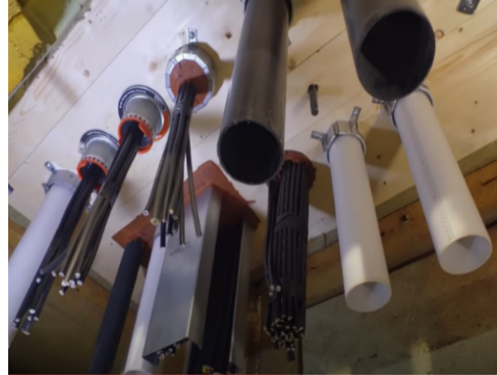
Figure 5-51: Photograph of a firestopping assembly of various electrical systems prior to testing
