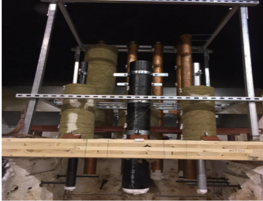
Figure 5-50: Photograph of a test assembly prior to testing with steel conduits (exposed side to the fire is below and unexposed side is above CLT structure)
