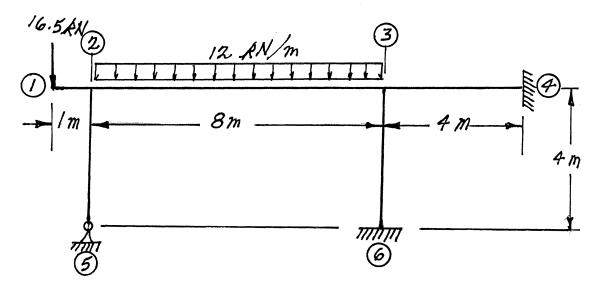
(22) 7. Use the **principle of virtual work** to calculate the vertical deflection at point 4 on the frame structure shown below. All members are inextensible and have the same EI value which is 2,000 kN.m<sup>2</sup>.
