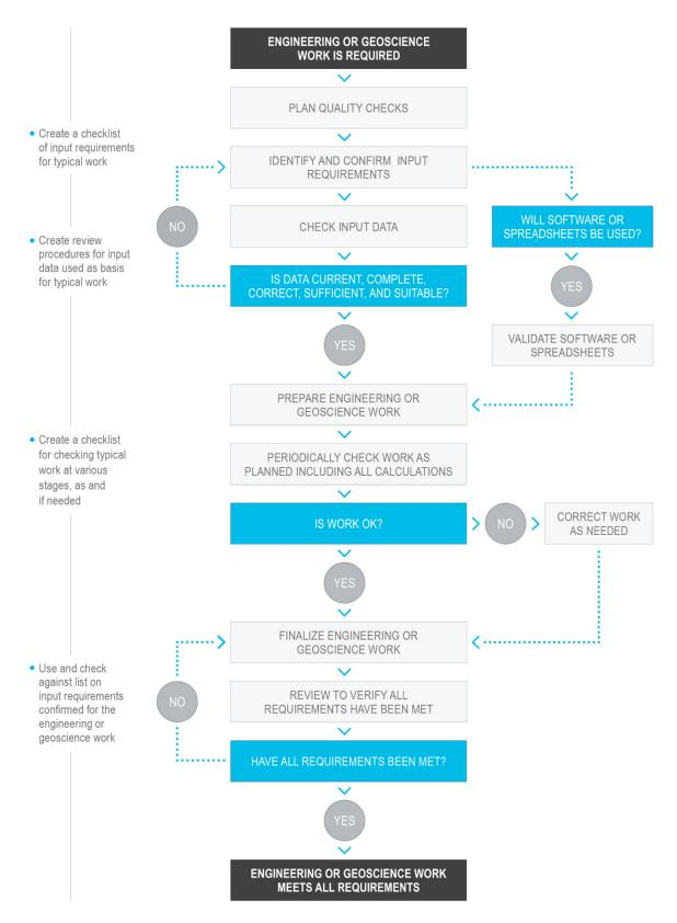
FIGURE 6-1: Example Checking Process Using a Flowchart and Checklists
