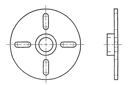
5. Sketch the steps that could be used to construct the following object using primitives (i.e., block, sphere, cylinder, cone, cylinder, prism, torus) using only Boolean operations (union, intersect, subtract).
