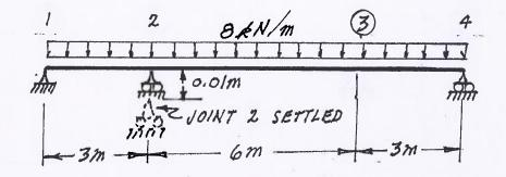
(24) 7. Using the slope-defection method or the moment-distribution method, analyse the structure shown below. Plot shear force and bending moment diagrams. On each diagram for each member, label the maximum and minimum ordinates (Minimum ordinates are frequently negative values). All members are inextensible and have the relative EI values shown on the structure.
