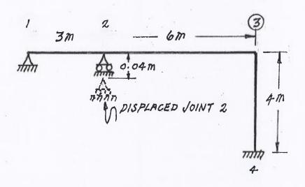
(18) 5. Use Castigliano's theorem (the "least work" theorem) to analyse the two-beam structure shown. Calculate and plot the shear force and bending moment diagrams for both beams. On each diagram, calculate and label the maximum and minimum ordinates (Minimum ordinates are frequently negative values). Both beams are inextensible and have the same EI value.
