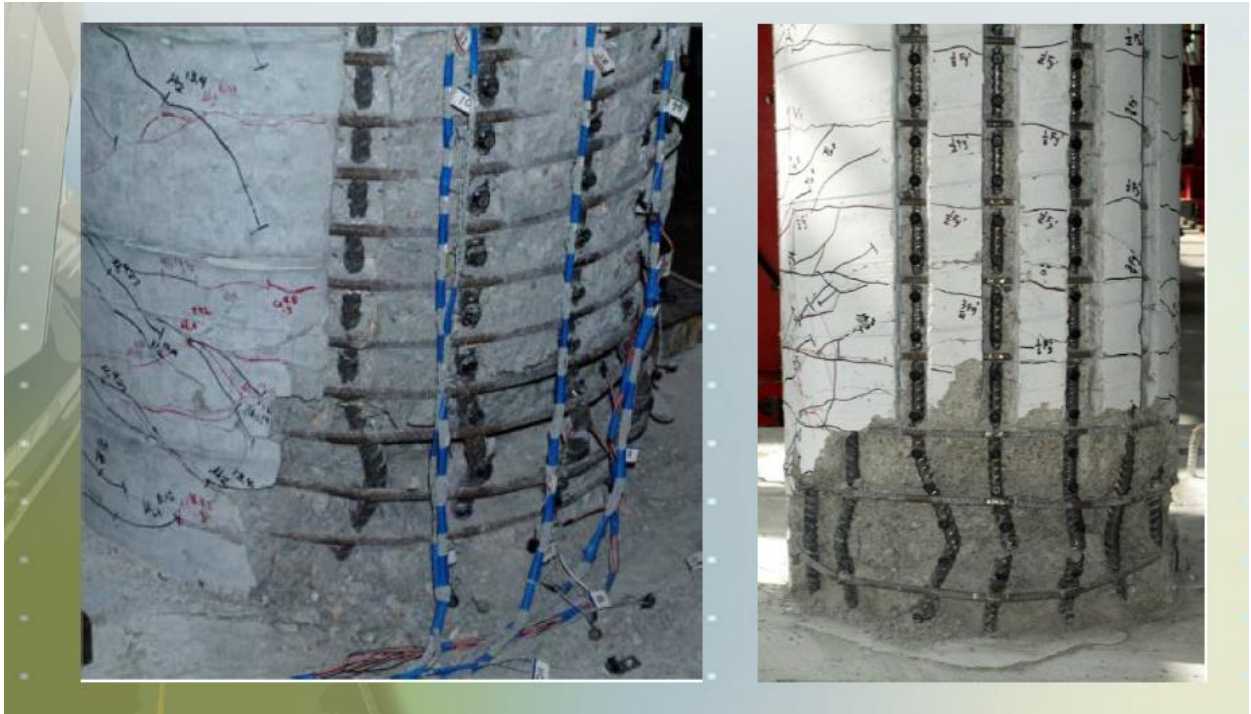
Extensive damage – Rebar buckling (Elmer E Marx, State of Alaska DoT)
