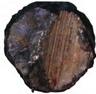
LEFT: This cross-section diagram of the haul rope estimates how each individual wire failed: black indicates cut-through wires, grey indicates partially cut wires, and white indicates wires that snapped without a cut from tension overload. DIAGRAM: TECHNICAL SAFETY BC. RIGHT TOP: This image is a cross-section photo of the Sea To Sky Gondola haul rope. The haul rope was organized in six bundles, each comprising 36 steel wires. Here, the bundles are labelled arbitrarily. PHOTO: TECHNICAL SAFETY BC. RIGHT BOTTOM: This wire was partially cut before it and remaining wires failed.
