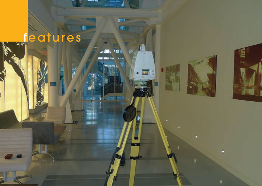
Above: Stationary Terrestrial Laser Scanner (TLS) on a tripod.
