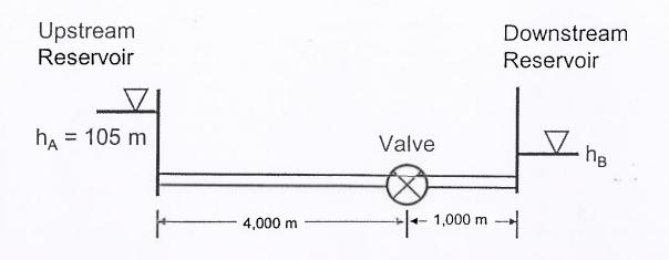
Figure 2. Schematic of water transmission system.
