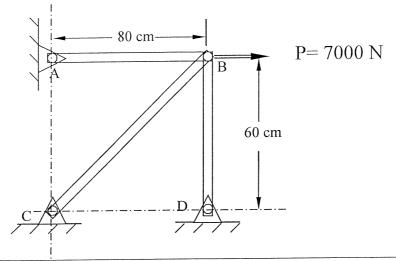
**2-** Using Castigliano's theorem, determine the displacement of point B of the beam shown below. Take E = 205 GPa,  $I = 165 \times 10^6$  mm<sup>4</sup>.
