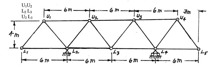
b) A vehicle, which is idealized as a uniformly distributed load over a length of 4 m, moves across the frame structure shown below. Calculate and show the influence line for bending moment immediately left of joint C. Also calculate the largest negative bending moment left of joint C. occurring while the idealized vehicle crosses the structure.
