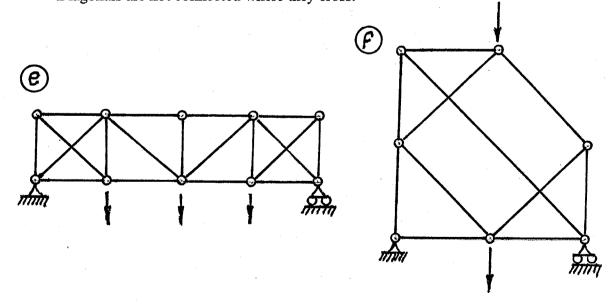
(18) 2. For each structure shown, compute the reactions and draw shear and bending moment diagrams. Indicate which are positive and which are negative segments of each bending moment diagram. For each shear and bending moment diagram, calculate and indicate the magnitudes of the maximum positive and maximum negative ordinates.
