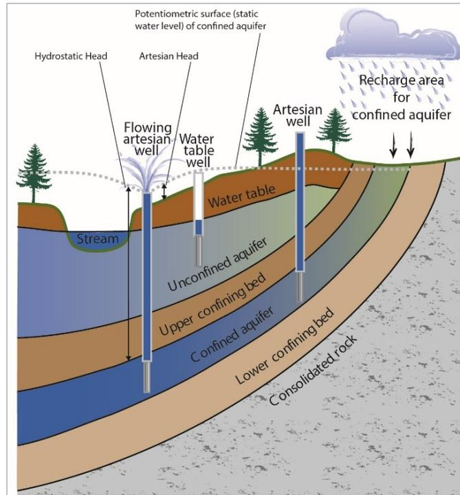
Figure 1: Geological and topographical controls affecting artesian and flowing artesian wells
