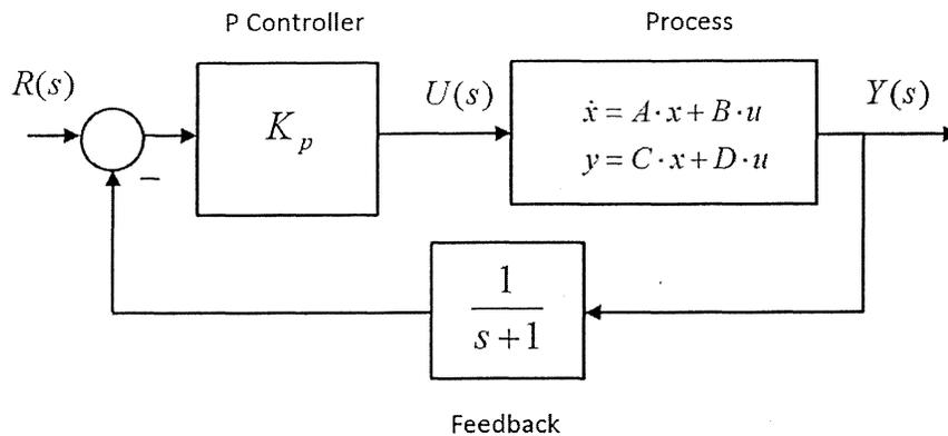
**Figure Q3.1** - Closed Loop System in Question 3
