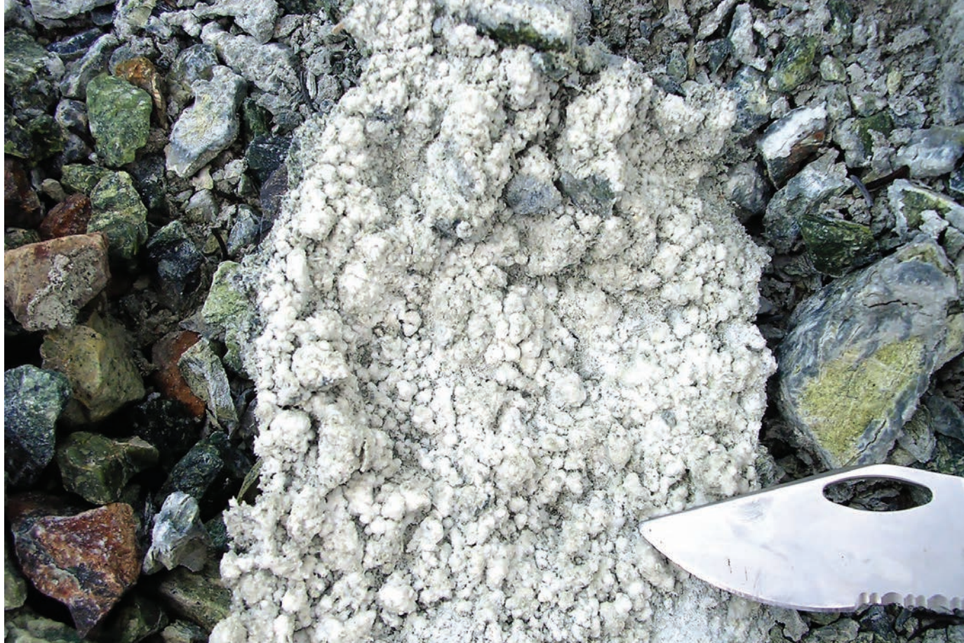
Magnesium carbonate crust on tailings of the closed Clinton Creek chrysotile mine, western Yukon, taken in 2005. PHOTO COURTESY OF UBC/GREG DIPPLE.
