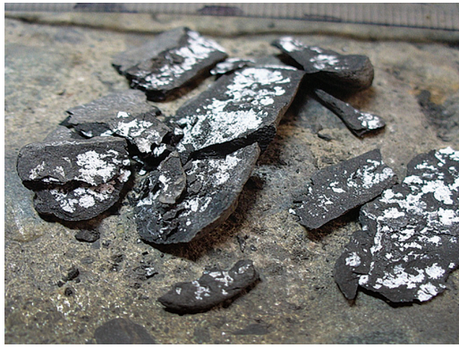
LEFT, FIGURE 5: Mudstone particle broken open to expose white gypsum crystals
