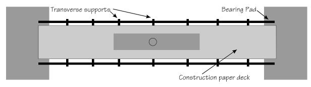
Figure 1b - Top view of bridge in testing apparatus
